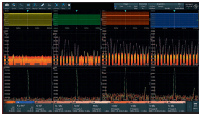
▲ Fig. 1 The R&S RTO6 displays the time and frequency responses of multiple channels simultaneously.
