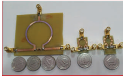
▲ Fig. 5 Classic Wilkinson power divider (left) vs. 2.5 GHz stub-loaded power dividers (right).
